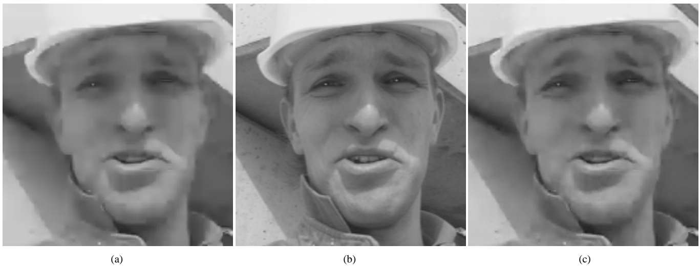
Fig. 4. Subjective comparison of the proposed technique in a region of the 51-st frame of the sequence Foreman. (a) Non-key frame. (b) Original frame. (c) Enhanced non-key frame. The sequence was encoded with Q_{key}=32 , Q_{non-key}=38 and GOP=4.
